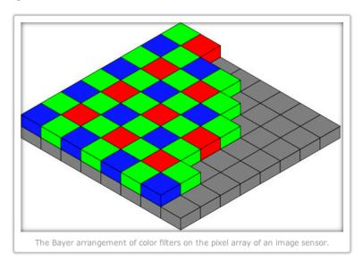
An image captured with a Bayer-filter camera is known as a Bayer pattern image. This raw sensor output must then be interpolated using demosaicing algorithms for the sensor to produce an accurate image, with full red, green, and blue image data for every pixel.
